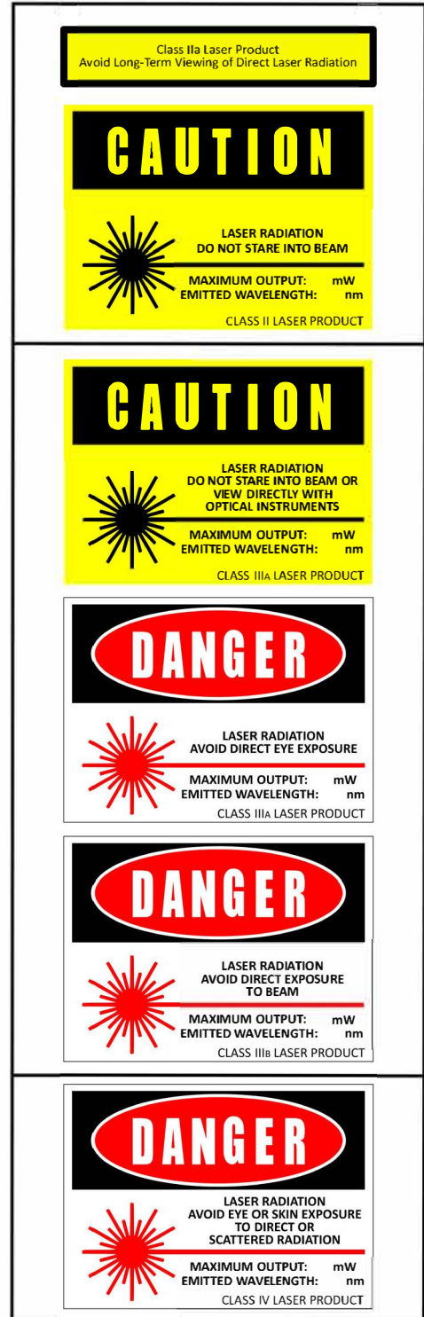
b) Class IIa to Class IV laser product warning markings according to the Food and Drug Administration (United States)
